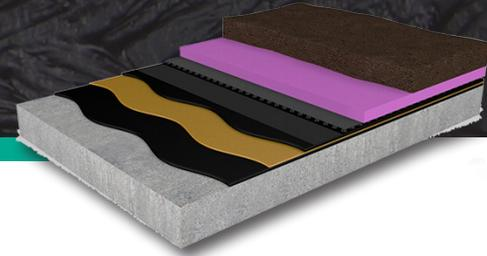
TREMPROOF® Dual Waterproofing System (DWS) is a dual membrane waterproofing system comprised of TREMPROOF TRA sheeting embedded into TREMPROOF 250GC. This unique waterproofing system is designed to have tenacious adhesion, long term durability, and remarkable chemical stability. The elastomeric properties of the system's components enable the complete assembly to withstand the most demanding waterproofing needs.
