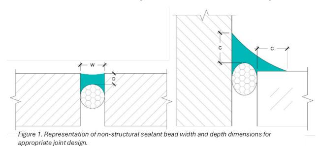
All non-structural sealant joints should be designed and installed in accordance with ASTM C1193 and ASTM C1472, represented in Figure 1 with the following labels:
