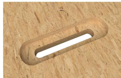
Available on any parapet cap configuration the oblong countersunk holes accept 1/2" (13 mm) diameter concrete anchors with up to a 1 1/4" (31.75 mm) washer. The oblong design is used primarily when "wet-setting" your anchors and are placed 24" (610 mm) on center and 6" (152 mm) from the ends of the 16' (4.8 m) board.
