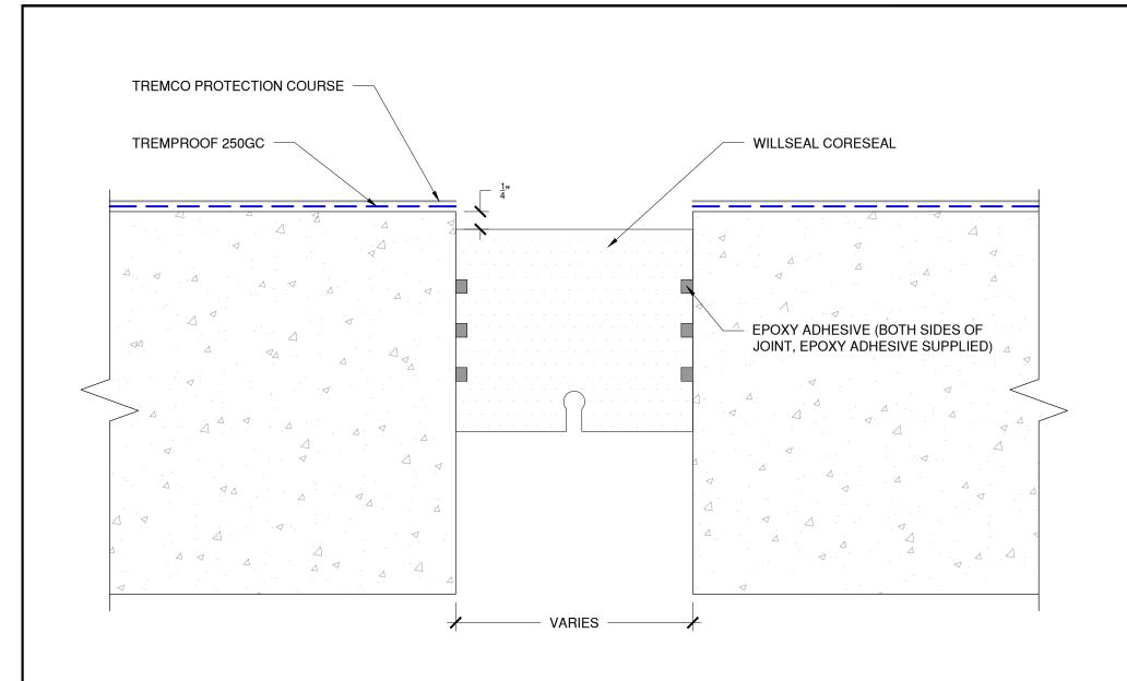
NOTE: REFER TO TREMCO'S PUBLISHED APPLICATION INSTRUCTIONS FOR ACCEPTABLE JOINT SIDE WALL SUBSTRATE CONDITIONS PRIOR TO INSTALLATION
