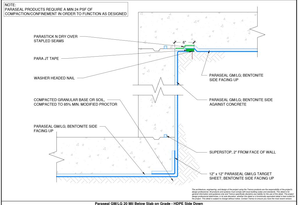
Detail: Paraseal GM/LG 20 Mil Below Slab on Grade at Elevator, Sump or Pit File Name:
