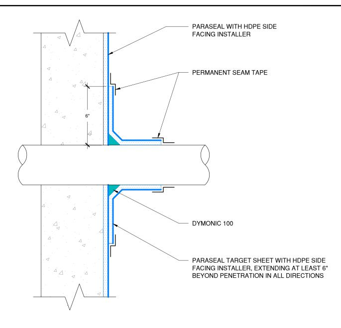
NOTE: PARASEAL PRODUCTS REQUIRE A MIN 24 PSF OF COMPACTION/CONFINEMENT IN ORDER TO FUNCTION AS DESIGNED
