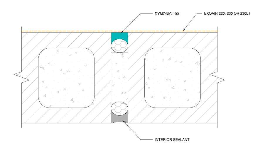
NOTE: JOINT TO BE FILLED AND ROLLED OR DOWEL TO SPAN BUILDING FACADE NOT SHOWN FOR CLARITY
