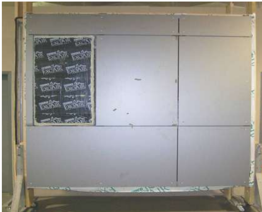
Photo No. 6 ExoAir 230 Perforated Wall with TRESPA TS110 Panel System
