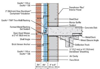
Note: ExoAir™ Primer is required for ExoAir™ 110 Vapor/Air Barrier
