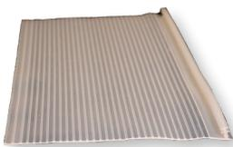
A pre-engineered silicone material used as a transition membrane for expansion joints between the Securock ExoAir 430 Panels. It is comprised of a flat, single-ribbed silicone extrusion that is adhered to the panel with Spectrem 1 silicone sealant.
