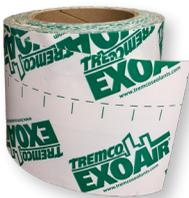
ExoAir 110AT is a 22-mil composite impermeable membrane that is comprised of 16 mils of butyl and 6 mils of HDPP facer. It is an impermeable, self-adhered sheet designed to be applied to exterior cavity walls to mitigate air infiltration/exfiltration, vapor transmission and water penetration.
