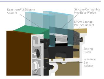
Complete glazing restoration systems from Tremco are available for a variety of applications. For the pressure bar system shown here, the original exterior gasket was replaced with Tremco's Silicone Compatible Headless Wedge and Spectrem 2 Silicone cap bead. Contact your local Tremco field representative or our Design Engineering Group for more information on our custom solutions.
