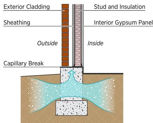
*Under similar conditions, air leaks can transport 50 to 200 times more moisture than diffusion. However, problems from vapor diffusion can build up and manifest over long periods of time.*
