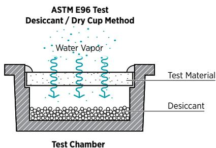
cup method and the standard water or wet cup method. The dry cup is designed to simulate a heated dry building during a high humidity conditions, simulating moisture drive into the building. The water, or wet, cup simulates vapor drive in the opposite direction, i.e. out of the building. Due to the differing vapor pressure differential, these test methods provide different permeance values for the same material.
