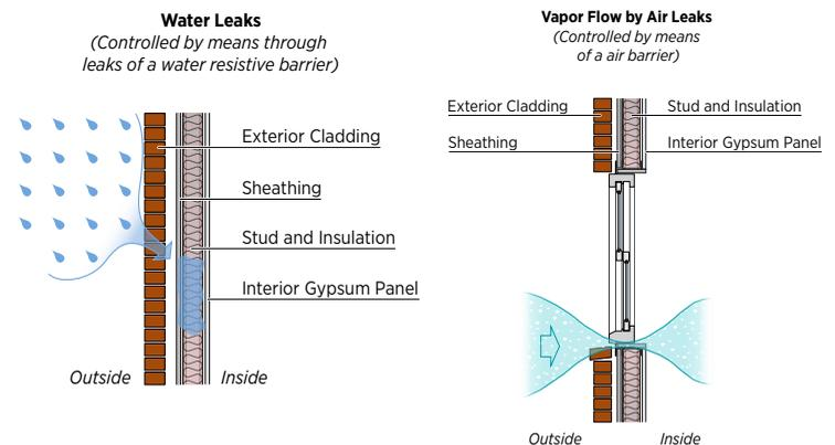
*Under similar conditions, air leaks can transport 50 to 200 times more moisture than diffusion. However, problems from vapor diffusion can build up and manifest over long periods of time.*
