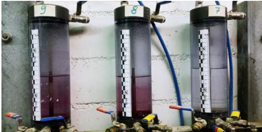
Fig.6: storage tanks for checking the flux of water
