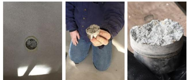
Figure 3 - Concrete substrate being pull tested failed prior to Tremco PUMA Primer, showing the primer's tenacious bond.
