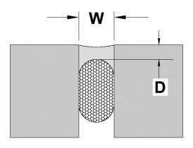
EXPANSION JOINTS - The minimum width and depth of any sealant application should be 1/4" x 1/4" (6 mm x 6 mm). The depth (D) of sealant may be equal to the width (W) of joints that are less than 1/2" wide.
