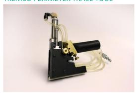
The Tremco Perimeter Trace Tool is used to cleanly apply spacer to the IG unit's glass perimeter, while precisely controlling start point, inset, and notch locations. The tool allows for **inside notching** that preserves integrity of the spacer's moisture vapor barrier allowing a wider range of applied perimeter sealant options.
