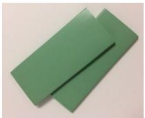
These solid silicone rubber pads protect the operator during hot-closing of sealant corners for the elimination of cold joints. Pads are sized at 1.5" wide x 3.5" long x 0.175" thick (38 mm x 89 mm x 4 mm) and are sold in boxes of 50 (Ref. Part #ENAPAD2 502).
