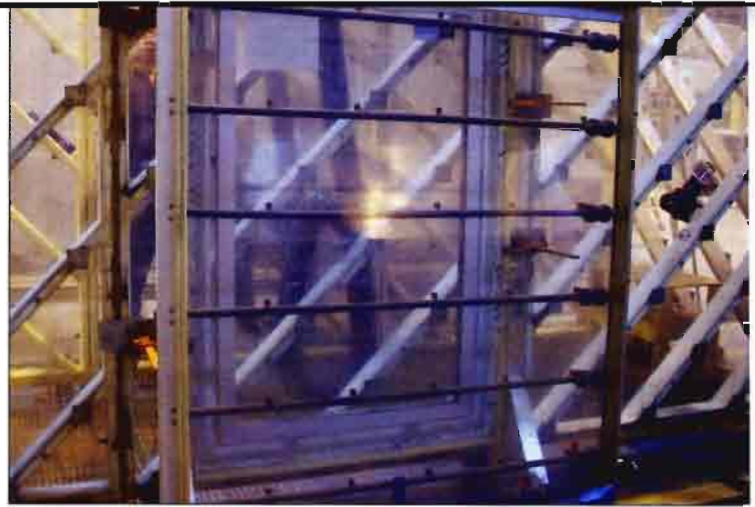
After an engineered transition assembly is tested for air penetration, a water spray rack is moved in front of the assembly. Water is sprayed at a prescribed volume while the window is subjected to negative air pressure (i.e. positive load), looking for any water penetration.
