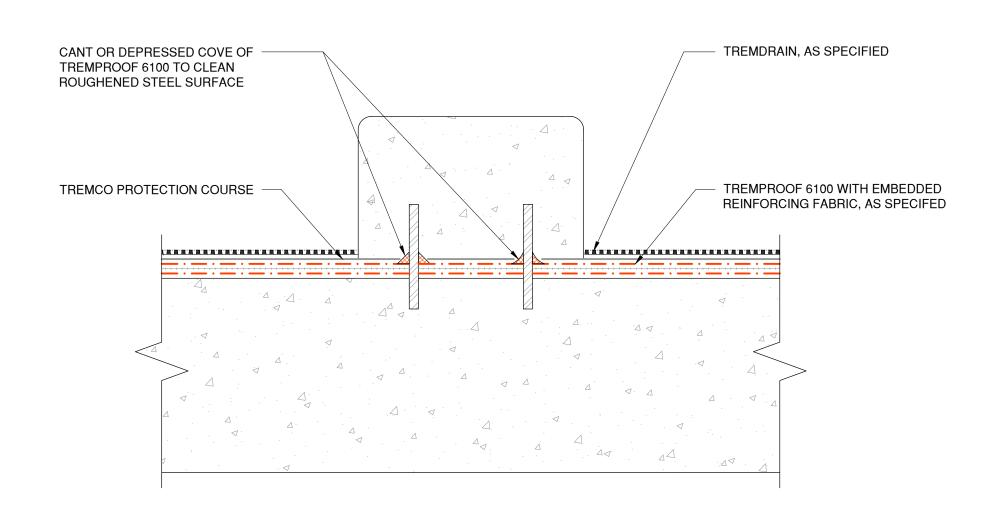
NOTE: TREMPRIME QD OR TREMCO APPROVED PRIMER MUST BE APPLIED BEFORE THE APPLICATION OF TREMPROOF 6100
