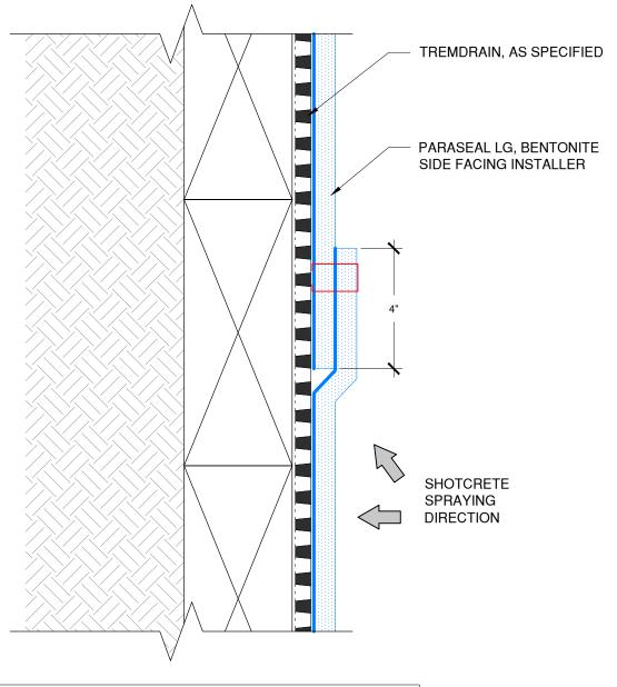
WHEN SPRAYING SHOTCRETE OR OTHER MATERIALS AGAINST PARASEAL LG, SPRAY EITHER DIRECTLY AT THE SEAM OR AT THE CLOSED EDGE OF THE SEAM SO AS NOT TO LODGE SPRAYED MATERIALS BETWEEN THE LAPPED SHEETS. NEVER SPRAY INTO OPEN EDGE OF SEAM.
