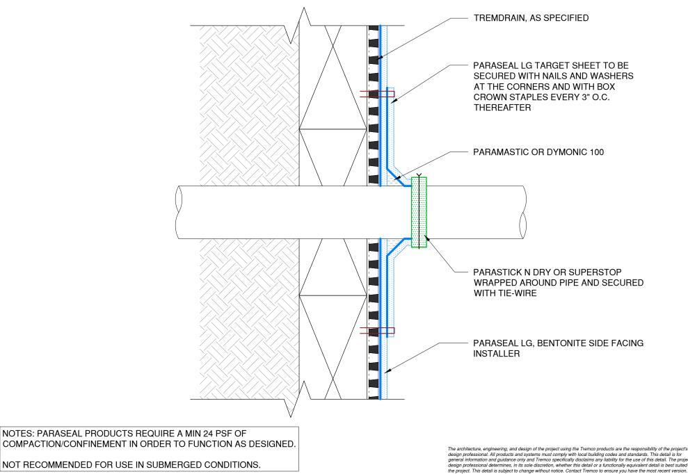
NOTES: PARASEAL PRODUCTS REQUIRE A MIN 24 PSF OF COMPACTION/CONFINEMENT IN ORDER TO FUNCTION AS DESIGNED.
