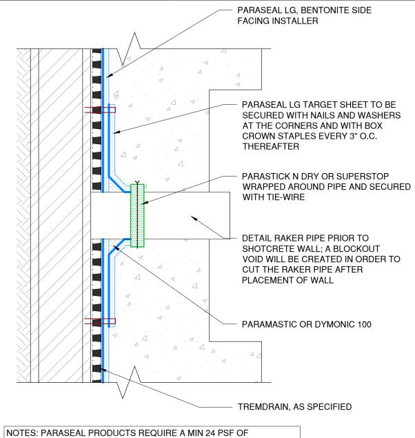
FILL CUT RAKER BLOCKOUT **VOID WITH CEMENT OR GROUT** FILL CUT RAKER PIPE WITH **CEMENT OR GROUT**
