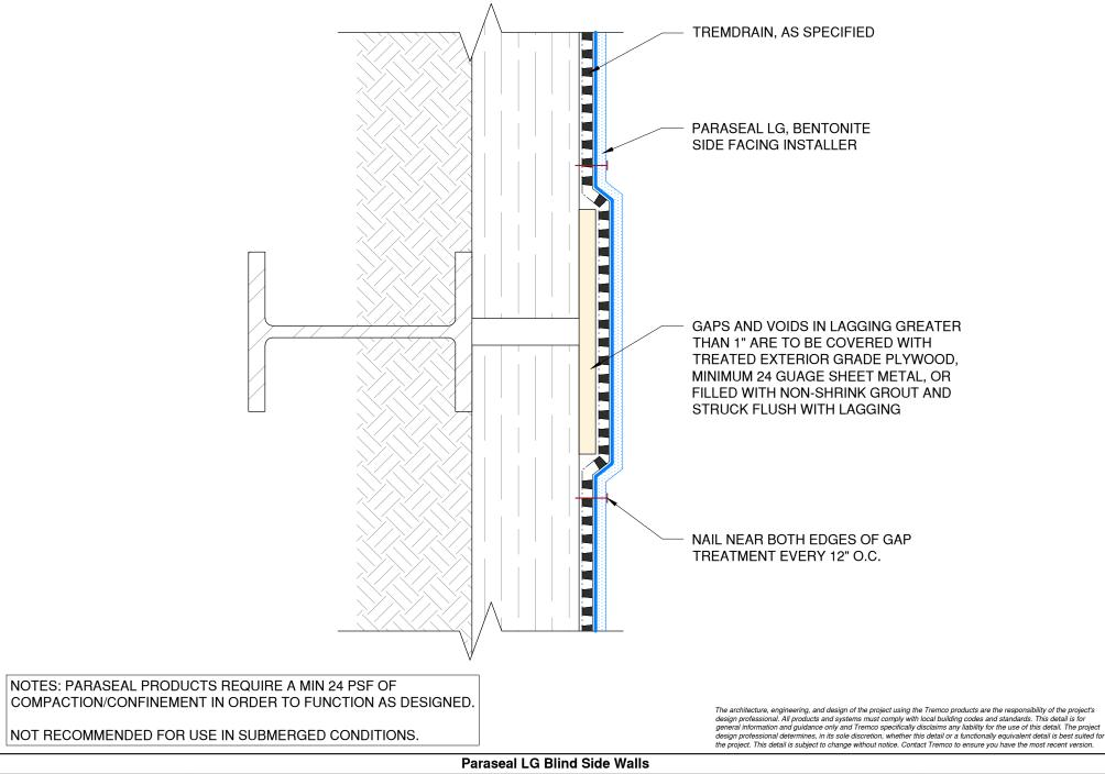
Detail: Paraseal LG at Transition over Gaps in Lagging
