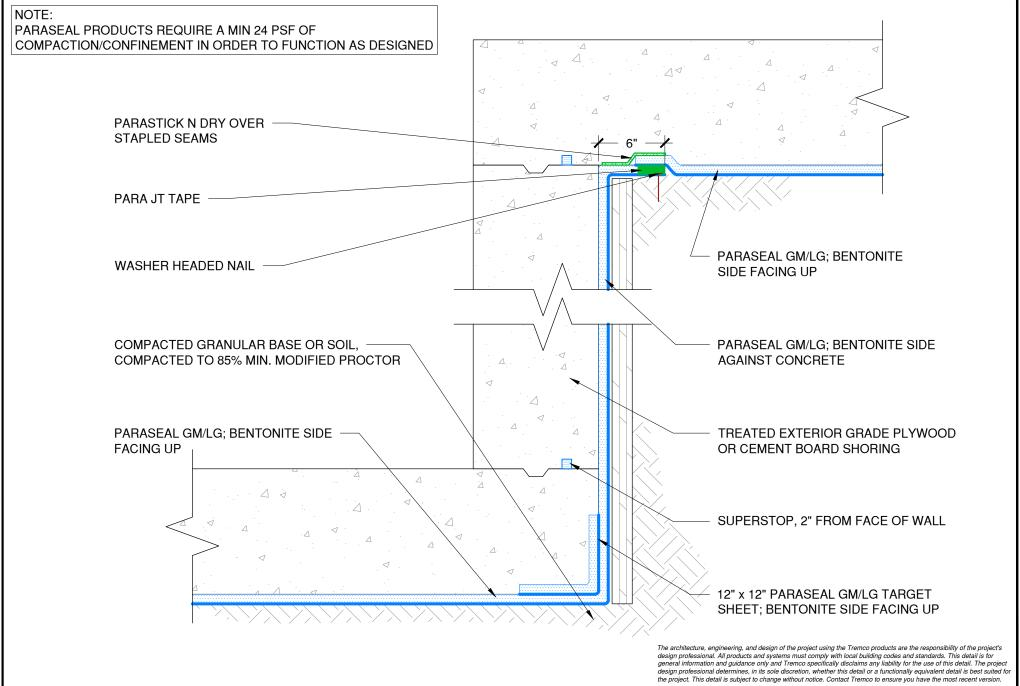
Paraseal GM/LG 20 Mil Below Slab on Grade - HDPE Side Down
