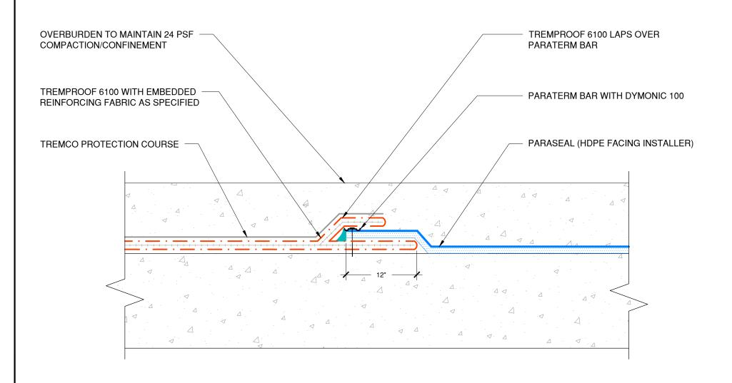
NOTE: PARASEAL PRODUCTS REQUIRE A MIN 24 PSF OF COMPACTION/CONFINEMENT IN ORDER TO FUNCTION AS DESIGNED
