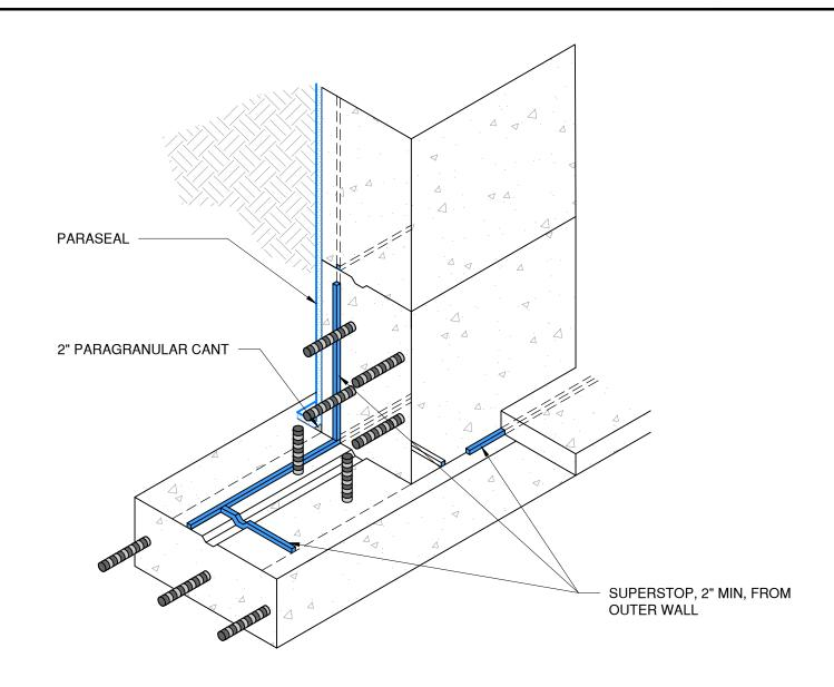
NOTE: PARASEAL PRODUCTS REQUIRE A MIN 24 PSF OF COMPACTION/CONFINEMENT IN ORDER TO FUNCTION AS DESIGNED
