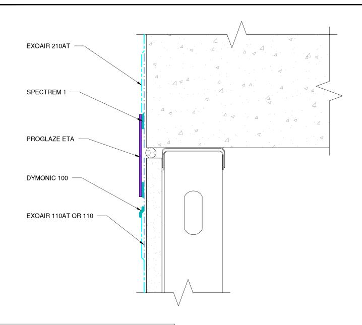
NOTE: BUILDING FACADE AND TOP OF FLOOR SLAB NOT SHOWN FOR CLARITY **EXOAIR PRIMER MUST BE USED WITH EXOAIR 110**
