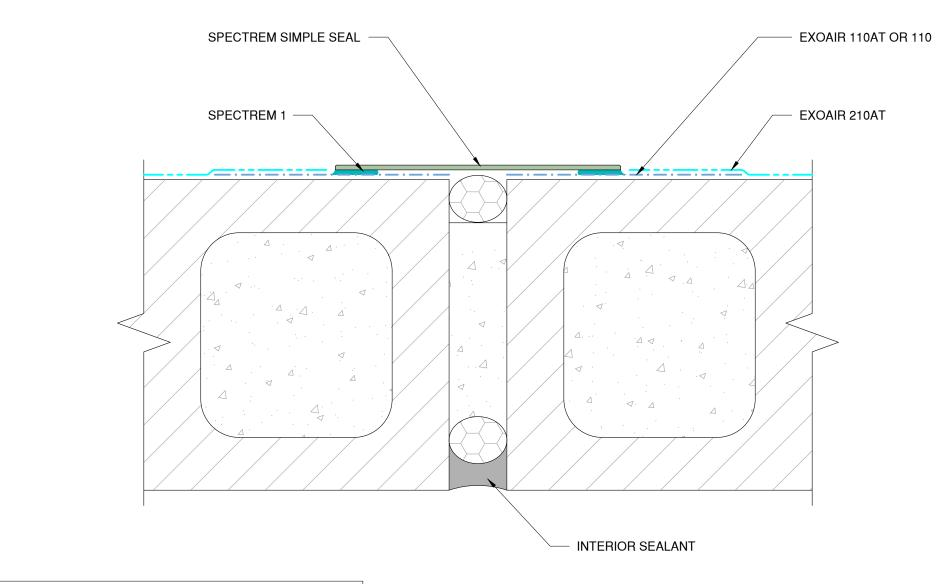
NOTE: JOINT TO BE FILLED AND ROLLED OR DOWEL TO SPAN BUILDING FACADE NOT SHOWN FOR CLARITY EXOAIR PRIMER MUST BE USED WITH EXOAIR 110
