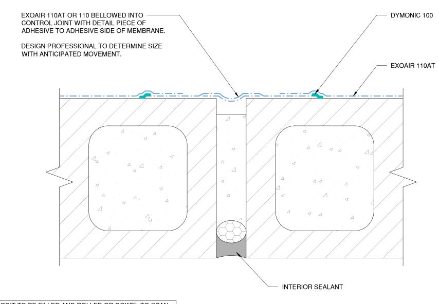
NOTE: JOINT TO BE FILLED AND ROLLED OR DOWEL TO SPAN BUILDING FACADE NOT SHOWN FOR CLARITY EXOAIR PRIMER MUST BE USED WITH EXOAIR 110
