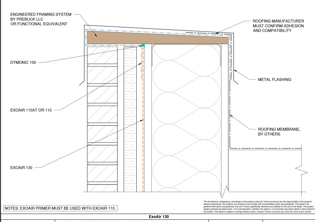
Detail: Impermeable Fluid - Roof Connection - Sheet Flashing
