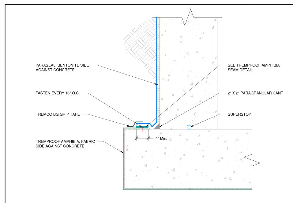
NOTE: PARASEAL PRODUCTS REQUIRE A MIN 24 PSF OF COMPACTION/CONFINEMENT IN ORDER TO FUNCTION AS DESIGNED
