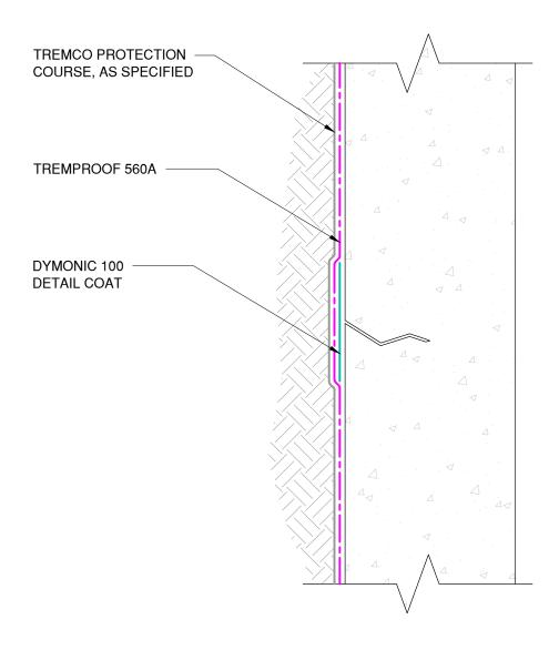
NOTE: TREMPRIME 500 MUST BE APPLIED BEFORE THE APPLICATION OF TREMPROOF 560A
