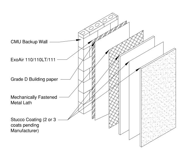
Detail: Stucco Isometric- Impermeable Sheet (Concrete)
