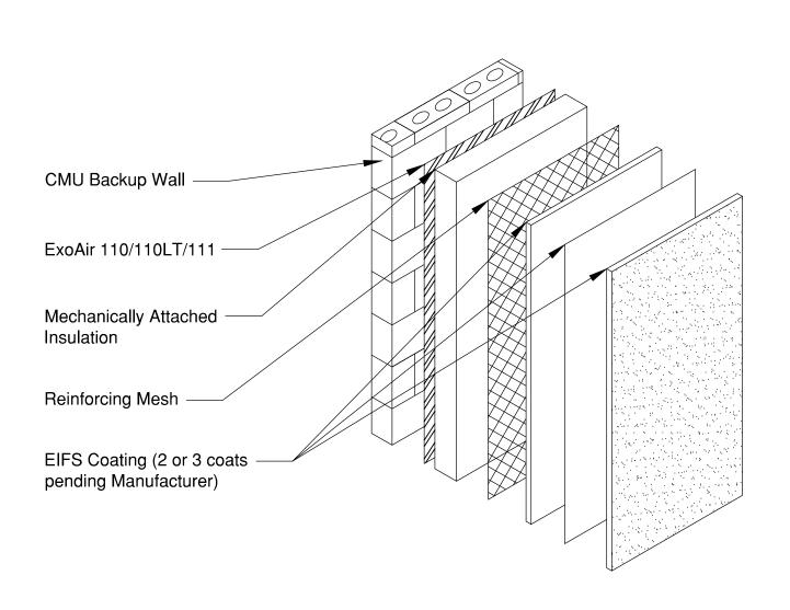
Detail: EIFS Isometric- Impermeable Sheet (Concrete)
