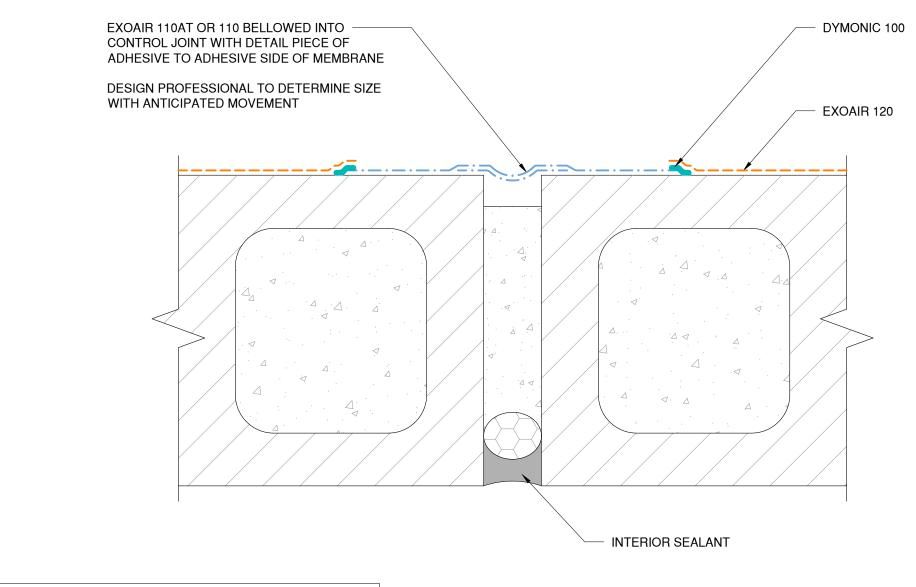
NOTE: JOINT TO BE FILLED AND ROLLED OR DOWEL TO SPAN BUILDING FACADE NOT SHOWN FOR CLARITY **EXOAIR PRIMER MUST BE USED WITH EXOAIR 110**
