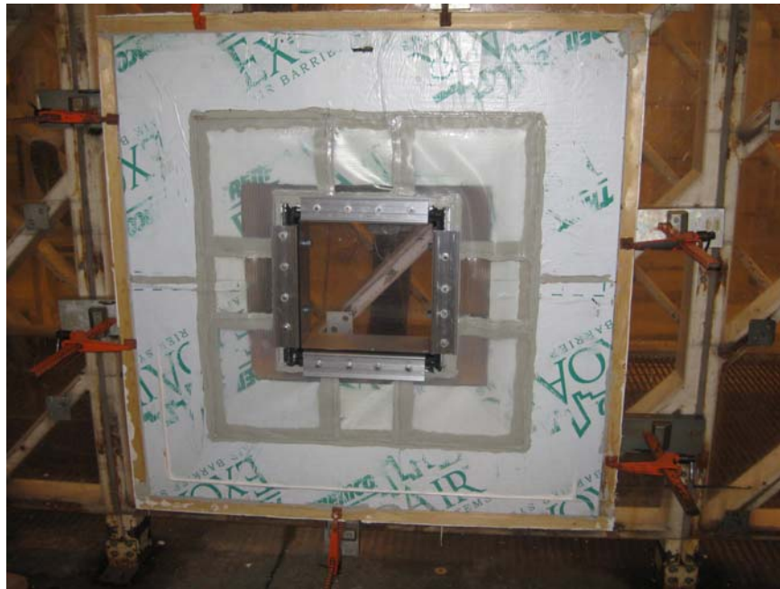
Photo No. 4 Structural Load Set-up
