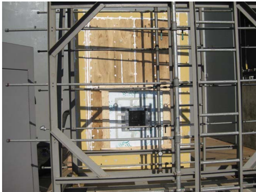
Photo No. 2 Water Penetration Set-up
