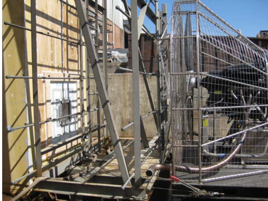
Photo No. 3 Dynamic Water Penetration Set-up
