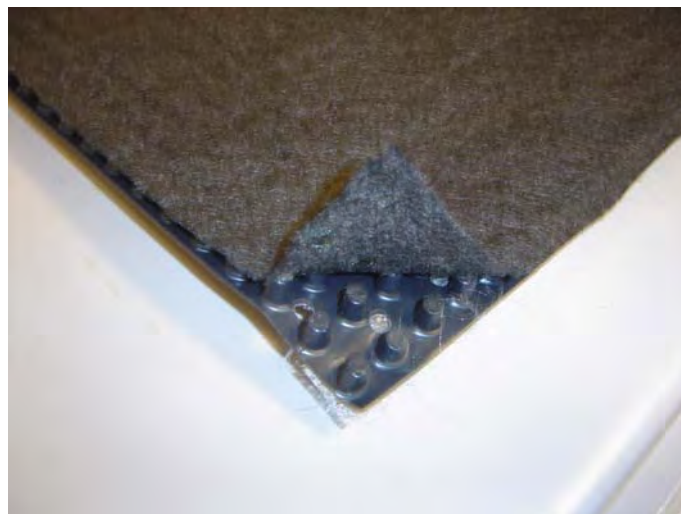
Figure 2: A Prefabricated Drainage Medium. Such a medium can be used to collect rainwater which can subsequently be used in the place of potable water for watering plants, flushing toilets and other non-potable applications.
